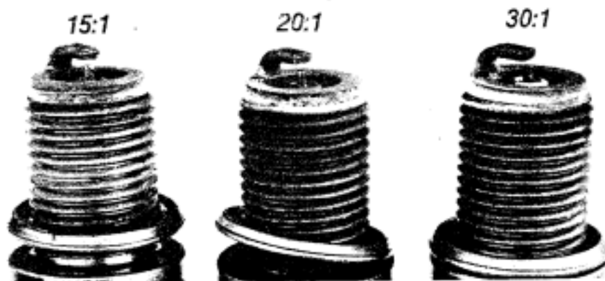
None of these plugs fouled; the one used in testing 15:1 premix did acquire a heavy coat of deposits.
